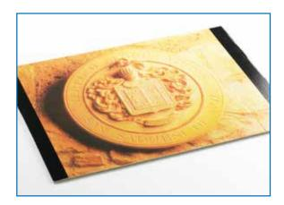
Full-coated paper; 4 colours + water-based varnish; 7500 sheets/h on Masterflex 160
