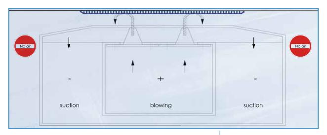
The principe of a drying unit
