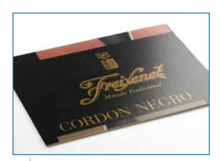
Full-coated paper; 5 colours + water-based varnish; 9000 sheets/h on Masterflex 160
